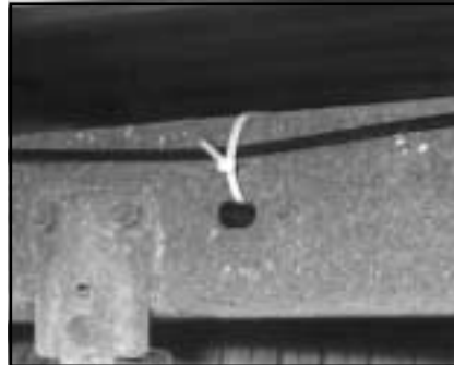
Inspect air lines to be sure it is not pinched. Tie straps may be too tight. Replace strap.
