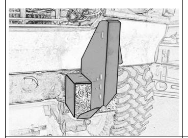
12. Fit the left and right hand bull bar mounting brackets to the appropriate chassis rails.
