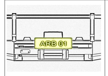
11. Fit the licence plate to the bull bar using two M6 x 16mm bolts, M6 flat washers and M6 flange nuts.
