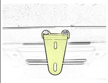
4. When fitting a low mount winch, fit the control box bracket to the bar. Fit using two M8 x 20mm bolts, M8 flat washers and M8 flange nuts.
