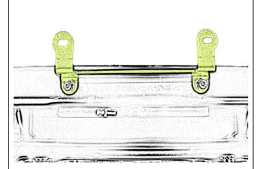
2. Fit the licence plate bracket to the bull bar using two M6 x 16mm bolts, M6 flat washers and M6 flange nuts.
