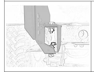
14. Fix the mounting bracket to the chassis using four ½" x 1 ½" bolts, eight ½" flat washers, four ½" spring washers and four ½" nuts. When happy with the alignment of the brackets tighten all the bolts.
