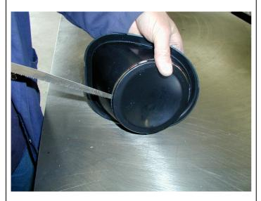
50. If no fog lights are not going to be fitted, fit light surround to bar as is. If fog lights are going to be fitted, cut out rear of surround using a key hole saw and remove rough edges with a file.
