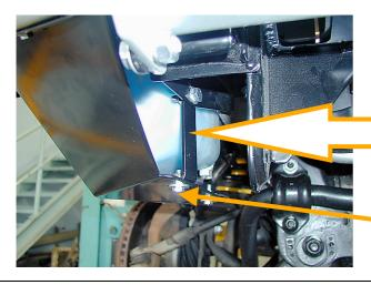
Fit 6mm hardware to bracket and guard Finger tighten
