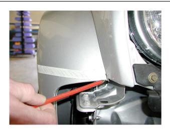
8. Mark a second datum point where the pencil is pointing, then using masking tape join the two datum points together making sure you have a level line.
