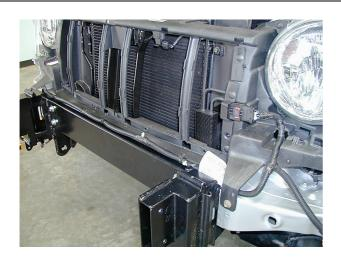
24. Refit vehicle loom to mounting system using cable ties and plug back into connector body.
