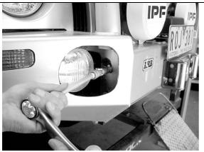
36. Slide bar onto vehicle mounting system and secure using 10mm hardware. Align bar with vehicle grille and flares, and tighten bolts using socket, extension and uni joint through fog light aperture in bar. Lastly retighten mounting system bolts when bar has been centralized sideways.
