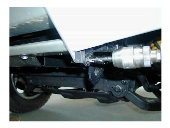
37. Once bar is secured to vehicle, using holes in locking plates as a template, drill 10mm holes through lower section of bar and bolt up using 10mm hardware.
