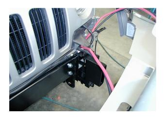
35. Position bar in front of vehicle and connect indicators, fog lights and fit winch cables under grille into engine bay close to battery.
