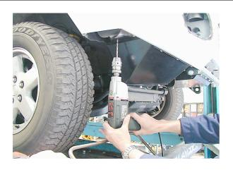
40. On RHS of vehicle, using vice grips to hold in place, drill a 6mm hole through washer guard into under side of vehicle crossmember and secure using 6mm hardware. When all bolts are fitted, tighten firmly. Cut plastic upward so you can tuck plastic inner guard in behind washer bottle guard.
