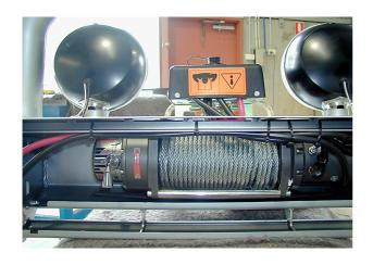
34. Cable tie power leads to battery, to the left side of the bar keeping clear of all moving parts.
