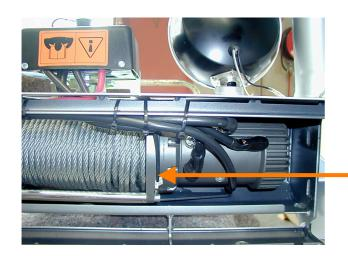
33. Cable tie power cables to bar keeping cables clear from all moving parts.
