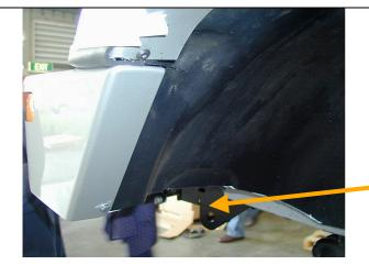
43. On the LHS of vehicle cut plastic inner guard as per photo, tuck in behind bar wing, secure to bar wing section using 6mm hardware.
