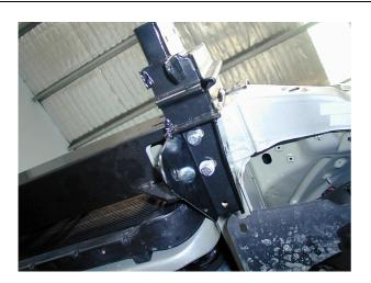
15. Fit 10mm hardware to the two most forward holes in lower brackets, to both sides of vehicle, making sure mounting system is hard up against vehicle crossmember, tighten firmly.
