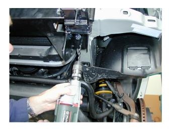
19. When front bolts are tighten, loosen off lower bolts in chassis brackets. Using a 10mm drill bit, drill out the most rearward hole in lower chassis bracket being careful not to drill too far into captive nut channel. When holes has been drilled, realigned the rear hole with rear nut in captive nut channel, and secure using 10mm hardware, then lightly tighten all bolts in lower chassis brackets.
