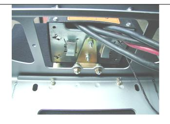
32 . Fit control box to control box bracket using original ¼" nuts from control box and connect power cables to winch motor as per winch instructions.
