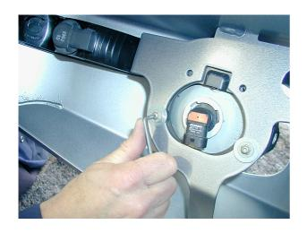
23. If bar is to have original fog lights fitted, position light into the two lower holes in light mounting bracket, place packer washer over light locating boss and refit light screws into all 3 holes, tighten firmly using torx key.
