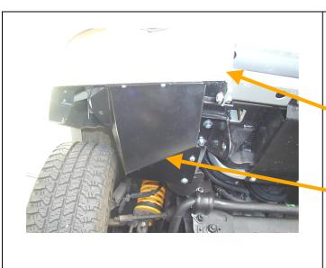
39. Bolt washer bottle guard to lower bar wing section using 6mm hardware. (finger tighten only)
