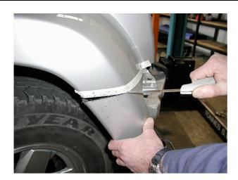
9. Using a key hole saw, carefully cut below the tape line.
