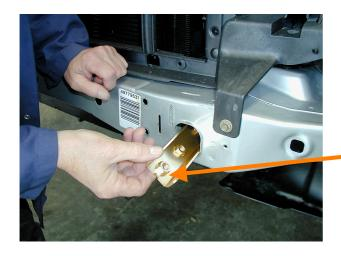
12. To fit mounting system to vehicle, fit captive nut channel in through front apertures in vehicle crossmember on both sides.
