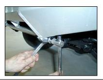
38. Fit washer bottle guard bracket to bar mounting system using 8mm hardware.
