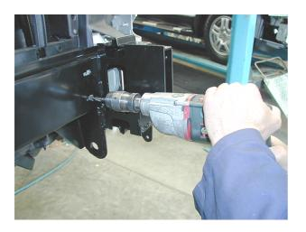
16. Using 10mm drill bit, drill out holes in centre of slots in front of crossmember.
