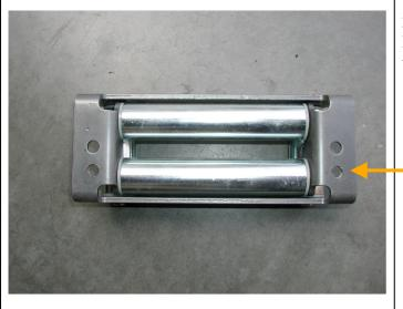
28. Drill 12mm holes under existing holes 25mm lower down the same pitch as existing holes, these will be the holes used to bolt to bar.
