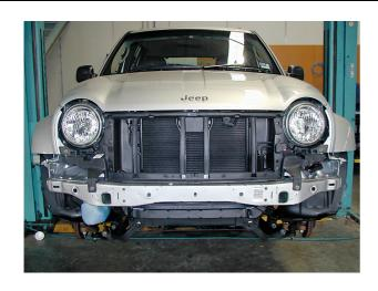
11. The vehicle is now ready to fit mounting system and bar.
