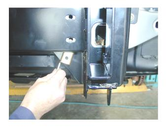
17. Once holes have been drilled, fit captive nut channels through lower aperture in vehicle crossmember.
