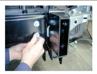
18. Secure using 10mm hardware and tighten firmly making sure mounting system is hard against vehicle crossmember.
