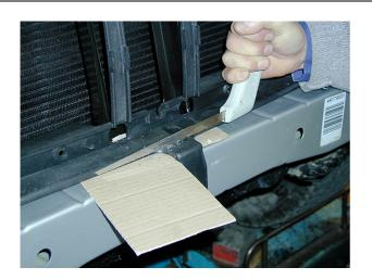
4. When bumper is removed, cut the lower plastic lug from grille panel to enable bull bar mounting system to bolt up against vehicle crossmember. Place either thick cardboard or plywood either side of lug to prevent paint damage.
