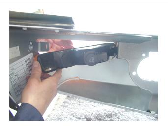
22. Indicator installation to bar, fit indicator tang into slot of fog light bracket and under outer bracket. Slide plastic packer between bracket and indicator and fasten using 4mm screw, flat washer and 4mm nyloc nut.
