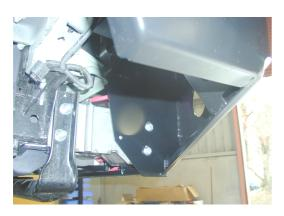
25. With assistance lift the bar into position and slide it over the two impact absorbers. Once in position bolt up the bar in the 8 places using the M10 bolts & hardware supplied, finger tight only at this stage.
