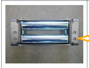
19. Drill out roller fairlead 25mm lower than original hole using a 12mm drill bit.
