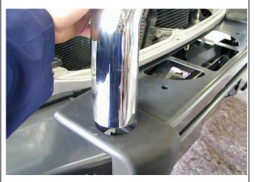
15. Fit the top tube through the hole in the top of the buffer and secure from underneath using M12 x 40mm bolt, spring washer and flat washer.
