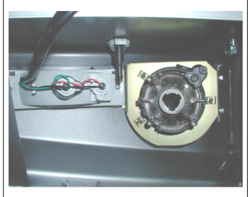
10. Fit the "u" nuts to the fog lamp bracket as shown, the nylon washer fits between the bracket and the lamp mounting foot (located on the adjustment side) fit the fog lamp with the screws provided.
