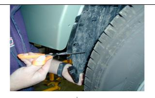
27. Trim the plastic inner guard liners by aligning with the bar and using the hole in the wing as a guide, drill a 6 mm hole and secure with the M6 hardware supplied
