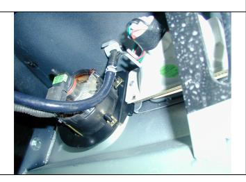
26.Re-connect the fog lamp harness and the turn signal harness on both sides of the vehicle, cable tie the wiring where appropriate.
