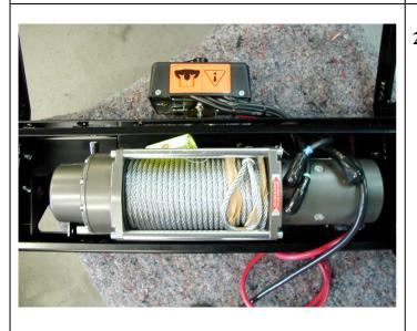
21. Fit winch into bar using 1 1/2" x 3/8" bolt on top holes and 1 3/4" x 3/8" bolt on the lower holes plus 25mm large flat washers and spring washers.
