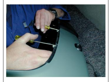
9. Placing the original bumper bar face down on a blanket remove all of the screws that hold the painted outer section to the main bumper. Using pliers remove the clip that holds the washer nozzle in the bumper and take out the nozzle (both sides). These are re-fitted into the bar once the fog lamp and turn signal are installed.
