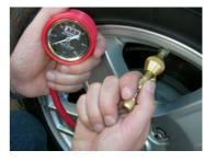
6. Remove the unit by turning the valve stem adaptor in an anti-clockwise direction.
