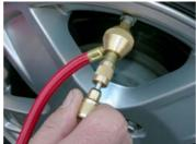
2. Push the valve core remover forward until it engages the valve and turn anti-clockwise to remove valve.
