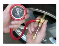
4. Pull out on the slide valve to release air. Push in on the slide valve to stop air and check the pressure. Note, gauge will not show correct pressure whilst deflating.
