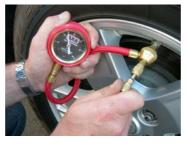
5. When the desired pressure is reached, push the valve core remover in and turn clockwise until the valve seats firmly. Note: Do not over tighten the valve core.
