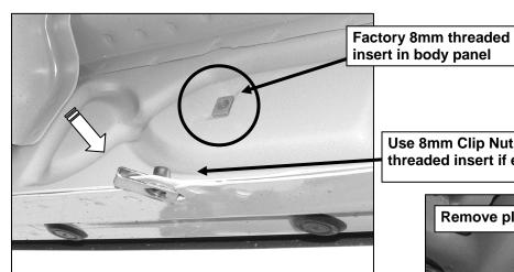
(Fig 1) Example of mounting location with factory threaded hole
