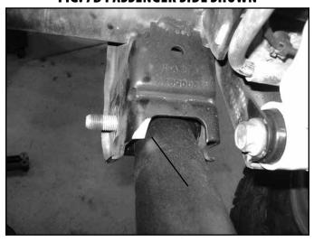
19. Using the OE hardware, install the arms so the bend is up and towards the center (Figure 8). The bend is centered. It may be necessary to raise or lower the axle to align the control arm bolts. Leave hardware loose, it will be tightened with the vehicle at ride height.
