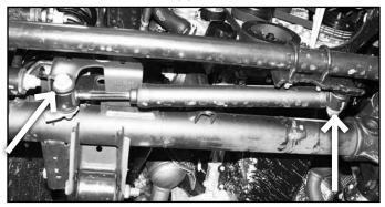
9. Disconnect the sway bar links from the axle and sway bar. (Fig 5)
