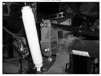
59. Position one of the new rear bump stop extensions over the support wing of the track bar bracket so that the existing holes in the factory bump stop pad are aligned with the holes in the track bar support and the bump stop. Fasten the bump stop and track bar bracket support to the factory bracket with 5/16" x 1-1/4" bolts, nuts and washers (BP 763). Run the bolts from the bottom up and torque to 25 ft-lbs. (Fig 23)
