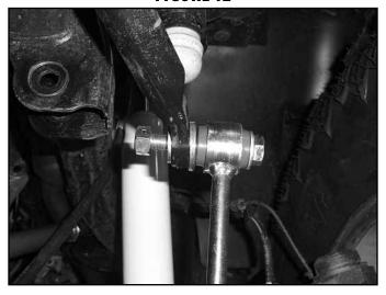
33. Locate the new sway bar link assemblies. Ensure that they are adjusted to equal length. The links should be adjusted between 8-1/2" and 8-3/4" from the center of the bushing to the very end of the disconnect. Do not lock off the jam nuts at this point.
