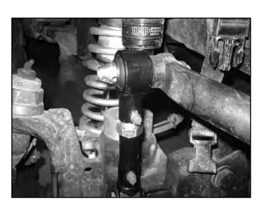
19. Locate the existing inner fender bolt up near the front body mount. Remove the bolt and attach the new lanyard to the inner fender with the bolt. Torque bolt to 10 ft-lbs. Slide the male clip up the lanyard and attach the female clip to it. This will be the stowed position for the lanyard when not in use. Do not wrap around the swap bar when the sway bar is connected.
