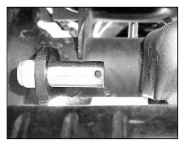
18. Place sway bar links onto pins, secure with click pins as shown. (Fig 4e, 4f)
