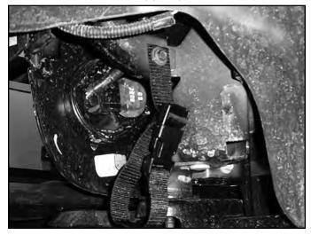
Note: The links must be completely removed from the vehicle when sway bar is disconnected and stowed in the vehicle with the retaining pins and spacers. Swing the sway bar up so that it is LEVEL and retain with straps. Do not drive the vehicle on-road with the sway bar disconnected.
