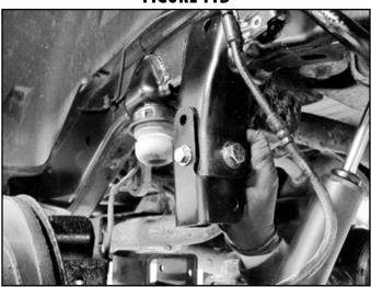
14. Reinstall the track bar bracket with the 9/16" hardware (BP 748) along with the provided crush sleeve (48) inside the factory mount. Run the bolt through the new bracket, OE mount and sleeve (Fig 12). Leave hardware loose.
