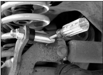
17. Attach the lower studs to the axle with included 1/2" nylock nuts. Tighten to 65 ft-lbs. The shortest stud will go on the Passenger's side, medium length stud goes on the Driver's side (Opposite for RHD vehicles). (Fig 4c, 4d)
