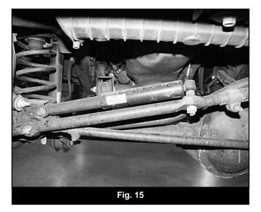
36. Disconnect the track bar from the axle (Fig 16). Disconnect the OE track bar frame bracket from the driver's side. Remove the four bolts/nuts and remove the bracket and track bar from the vehicle. Save the frame mount hardware.
