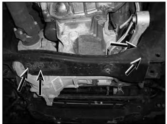
22. Inspect the inside factory control arm mounting holes. There will be a sharp lip left from the original control arm/hardware. Use a file or rotary grinder to remove the sharp lip left from the control arms (Fig 10). This will allow the new cross members to be installed easily.
