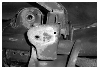
27. Locate the new provided bump stop brackets (02199). Place a bump stop bracket up to the original mount and line up the center of the two slots with the two holes in the factory mount. Using the third slot in the bracket as a guide, mark the center position to be drilled (Fig 14). Remove the bracket and drill a 7/16" hole at the mark.
