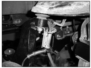
42. Install the provided offset sway bar link u-bracket (02102) on the lower control arm in the original sway bar link hole with a 5/8" x 1-3/4" bolt, nut and washers (BP 569). Position the bracket so that it offsets in toward the center of the vehicle (Fig 26). In some cases it may be necessary to slightly clearance to hole for the 5/8" hardware. (4wd model shown - 2wd similar)
