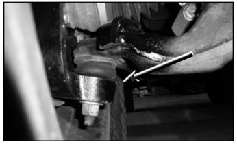
6. To determine the Z-height use the following equation: Y-X=Z. For the intended 7" of lift the value for Z should be approximately 4". If your value for 'Z' is less then 4" the torsion bars need to be adjusted up (tightened). If your value for 'Z' is more then 4" the torsion bars need to be adjusted down (loosened). These values are for reference but should not vary more then 1" in either direction.
