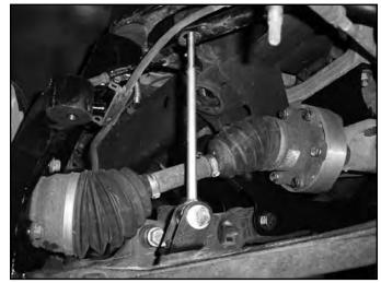
44. Install a provided stem washer (S100776) followed by a stem bushing (SB26BK) on each sway bar link. Install both links into the sway bar and install a second stem bushing followed by a second washer. Fasten the sway bar link upper assemblies with 3/8" nylock nuts (BP 569). Leave nuts loose (Fig 28).
