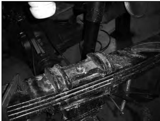
44. Remove the factory lift block. It will be reinstalled later.
