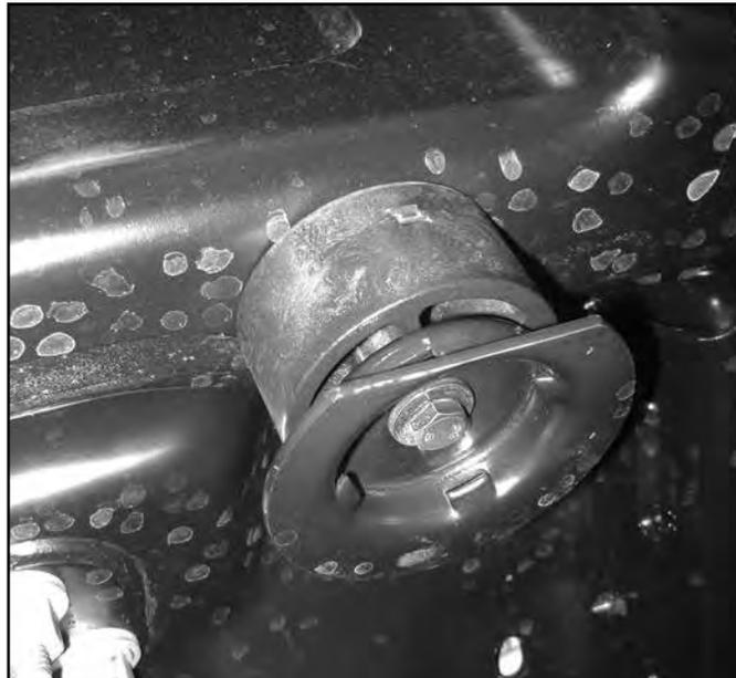
19. Grease the bump stops and reinstall into the factory cups. Raise the axle to get the bump stops to press into the cups. (Fig 11)
