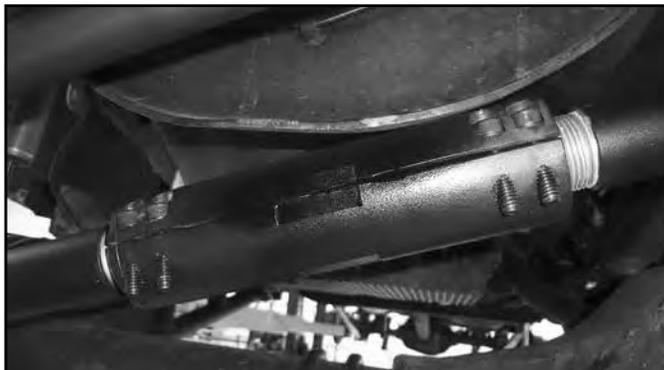
35. Adjust steering wheel to center, this will require lengthening of the drag link. Do not drive the vehicle with the steering wheel off-center for extended distances / speeds or a trip to the dealership may be required to reset the computer. Note: if there is less than 1-3/4" of thread engaged in the adjusting collar, the track bar must be shortened to allow for adequate thread engagement of the drag link.
