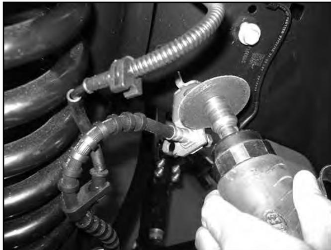
11. Disconnect the shocks by removing factory hardware (Fig 6a, 6b). Retain lower bolt and nut tab for later reinstallation.
