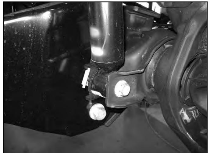
12. Disconnect sway bar from the frame. Retain (4) mounting nuts. (Fig 7)
