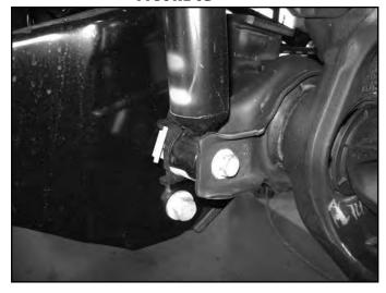
12. Disconnect sway bar from the frame. Retain (4) mounting nuts. (Fig 7)
