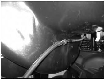
8. Remove the brake line bracket from the lower coil seat. Retain hardware. (Fig 3)
