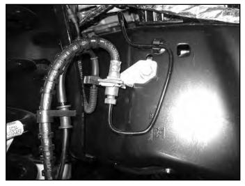
10. Carefully cut the factory bracket so that the brake line can be removed without breaking loose the fittings. Remove the factory brake lines from vehicle. Do not damage the brake line! (fig. 5)
