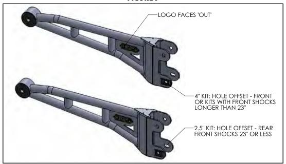
16. Tighten the radius arm hardware at the axle to 222 ft-lbs. Do not tighten the pivot bushing at the frame. (Skip ahead to bump stop installation)
