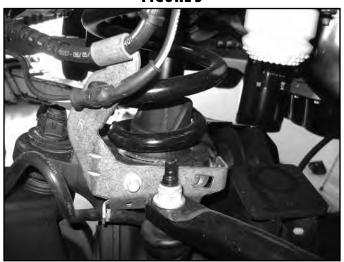
9. Disconnect the brake line bracket frame (Fig 4). Retain hardware.
