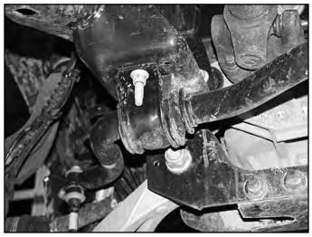
Carefully remove the hub dust cap to expose the axle shaft nut (Fig 7 & 8). Remove the nut. Retain the cap and nut, they will be reinstalled
