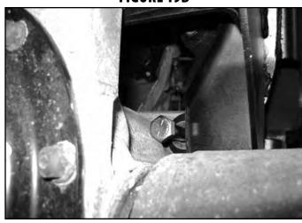
31. Fasten the support bracket to the rear of diff drop bracket. Fasten with the driver's side rear cross member hardware. Attach the hardware at the differential bracket from the front to rear. Leave all hardware loose at this time. (Fig 20A).
