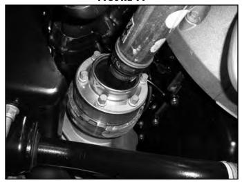
23. Remove the passengers side CV only. Strike the shaft with a hammer to dislodge it from the splines. This will make handling the differential much easier. (Fig 12)
