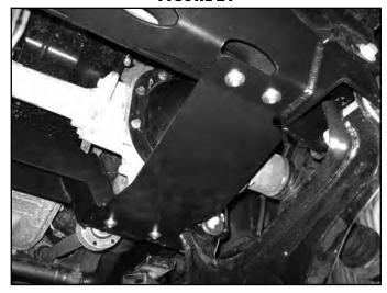
38. Attach the sway bar drop brackets with new 3/8" x 1-1/4" bolts, washers and nuts. Run hardware from bottom - up, snug but do not tighten at this time.
