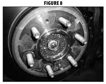
14. Loosen but do not remove the three strut assembly mounting nuts at the frame (Fig 8). Do not loosen the middle strut nut.
