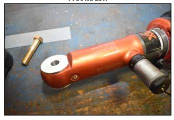
43. Install the strut spacer assembly to the strut / coilover using the provided 3/4" bolt, washer, and nut (BP 883) through the spacers. Leave hardware loose. Apply the clear decal around the body of the strut / coilover in the location where the strut clamp will go around the body. Figure 23B. This will create a barrier between the aluminum and steel to prevent any corrosion. Make sure the strut spacer installed as shown, the strut spacer has an offset built into it for clearance.
