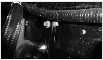
83. Install the provided spacer washer between the rear differential and rear brake line bracket attaching the with the 5/16" bolt and washer (BP #883) and thread locker. (Fig. 38) Tighten hardware to 209 In-lbs.
