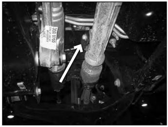
25. The driver's side rear lower control arm frame pocket must be modified to provide clearance for the differential in its relocated position. On the front side measure from the inside edge of the slot 3/4" (Fig 14A & B). Make a vertical cut line at the mark.
