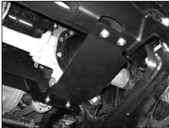
42. Attach the sway bar drop brackets to the frame using the factory nuts and nut tabs. Snug but do not tighten at this time.
