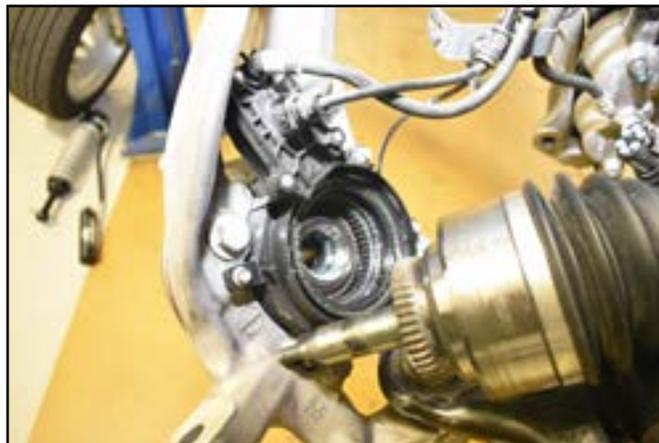
17. Loosen but do not remove the upper and lower ball joint nuts (Fig 10A / B). Unseat the upper and lower ball joints from the knuckle, refrain from hitting the aluminum steering knuckle, use appropriate tool to separate ball joints, avoid damaging the threads.
