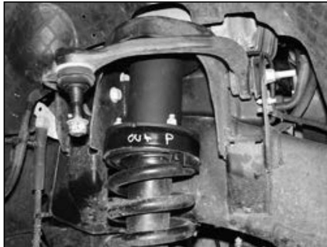
47. If installing Fox Coilovers, install the coilover the same as the factory strut using the provided hardware with the coilover. Install the reservoir mount to the top of the strut bucket on the frame. Attach the reservoir to the reservoir mount using the provided clamps.
