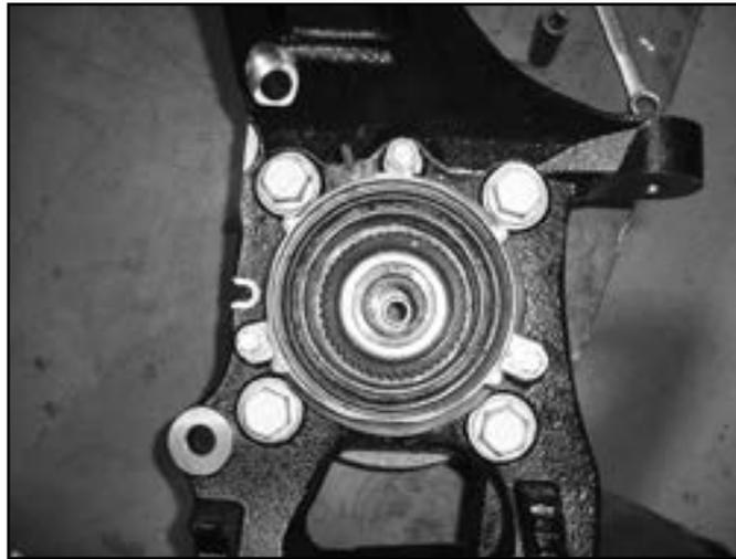
51. Install the new knuckle assembly on the lower control arm ball joint and loosely fasten with the original nut. Install the CV shaft in the hub, swing the whole assembly up and attach the lower control arm to the strut with the original hardware (Fox coil-overs use included hardware). Leave all hardware loose.
