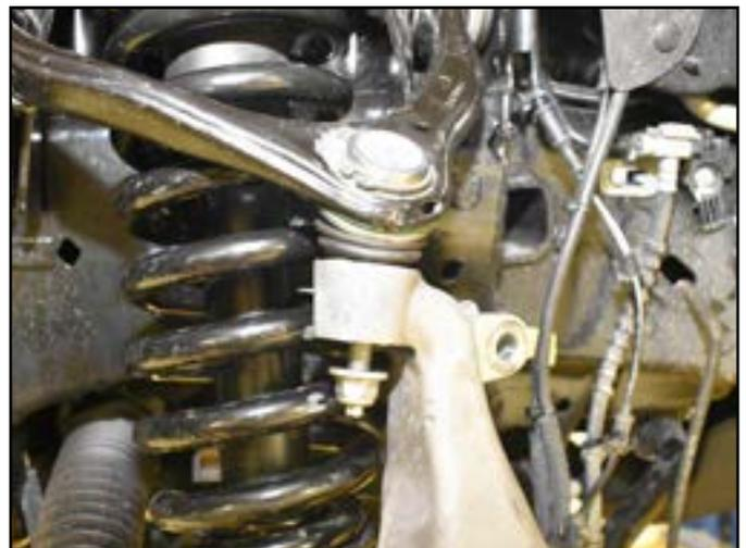
18. Remove the upper ball joint and the strut-to-lower control arm hardware. Swing the knuckle/lower control arm down to remove the CV shaft from the hub. Retain ball joint nut and strut bolts.
