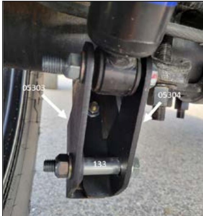
92. Attach lower shock with factory hardware, snug hardware but do not tighten at this time.
