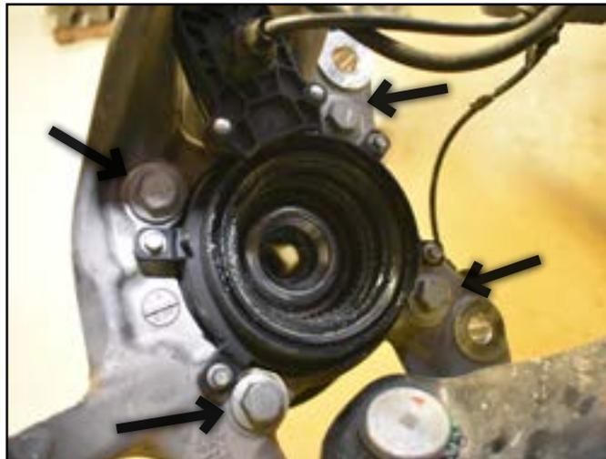
49. Install the hub into the corresponding new BDS knuckle (Driver- 03991, Passenger- 03992) and fasten with the OE bolts. Make sure the ABS wire is located at the 'top' of the hub. Use thread locker on the bolt threads and torque to 129 ft-lbs.
