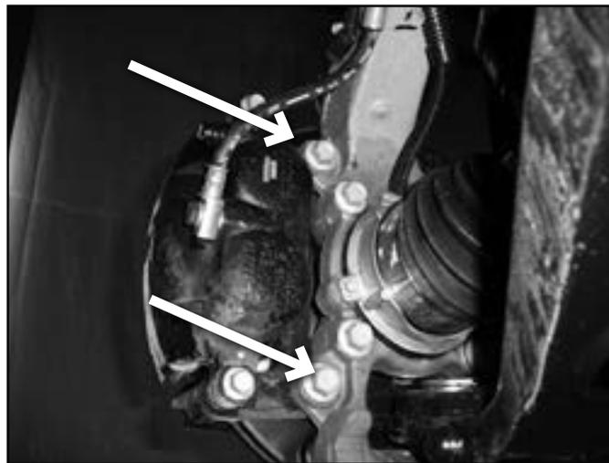
7. Remove the brake rotor and set aside.
