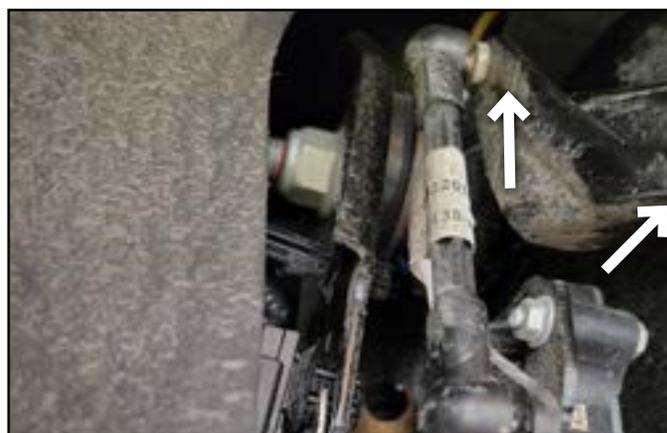
66. Install the supplied sensor relocation brackets (05305 Driver Side, 05306 Passenger Side) to the upper control arms with factory bolts. Torque to 177 in-lbs. Reconnect sensor linkage to the relocation bracket with the factory nut. (Fig 34. Driver Side Shown)
