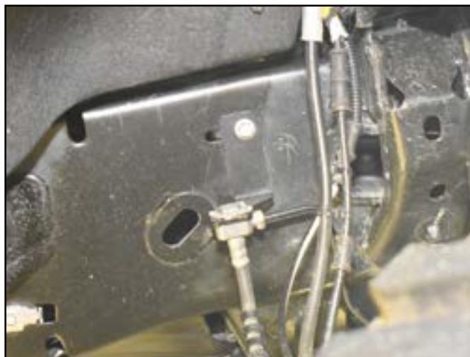
60. Install the dust shield with the factory 6mm bolts, tighten bolts to 133 in-lbs.
