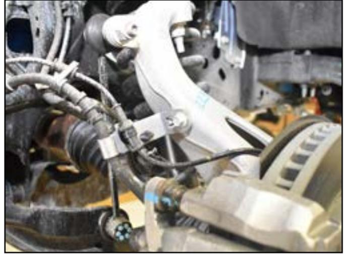
11. Disconnect the tie rod ends from the steering knuckles. Remove and save the nuts. Avoid hitting the aluminum steering knuckle, use appropriate tool to remove tie rod end from steering knuckle. Take care not to strike the tie rod end, or damage the threads (Fig 5).
