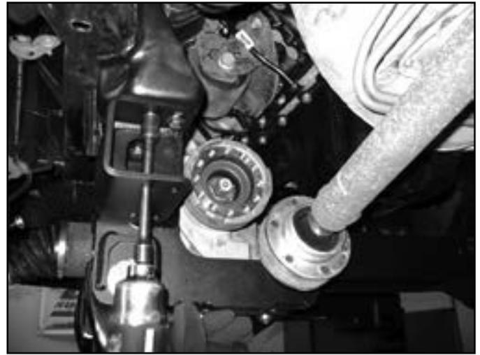
43. With the lower control arms installed torque the four cross member mounting bolts to 250 ft-lbs. Ensure that the front cross member is centered in the vehicle. Torque the differential skid plate bolts to 65 ft-lbs. Tighten sway bar drop hardware to 46 ft-lbs.
