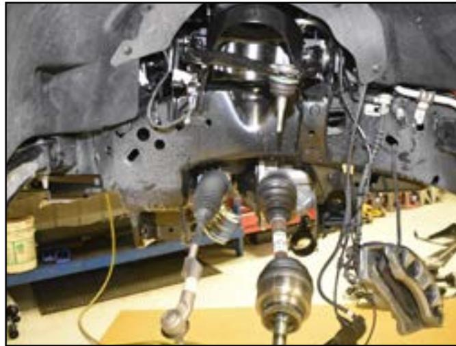
24. Take a wire brush and remove the material from the threads of the four bolts that attach the OE rear cross member. Remove the bolts and cross member from the vehicle. Discard the cross member and hardware (Fig 12).
