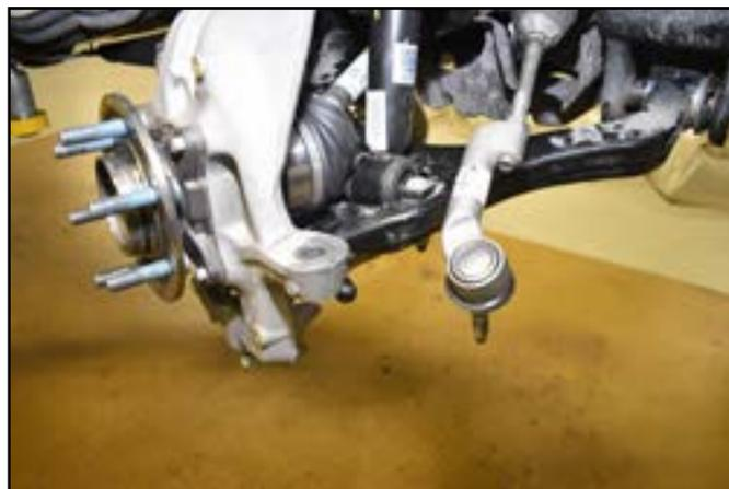
12. Disconnect the sway bar links from the steering knuckle (Fig 6A). Retain hardware. The sway bar links do not need to be removed from the sway bar.
