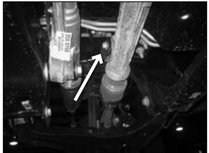
28. The driver's side rear lower control arm frame pocket must be modified to provide clearance for the differential in its relocated position. On the front side measure from the inside edge of the slot 9/16" (Fig 16A / B). Make a vertical cut line at the mark.
