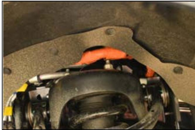
16. Remove the 4 bolts attaching the 4wd actuator hub assembly to the steering knuckle. Figure 9 is shown with the CV shaft pulled out for clarity. Note that some models starting in 2022 will not have the 4wd actuator hub assembly, skip this step if not equipped.
