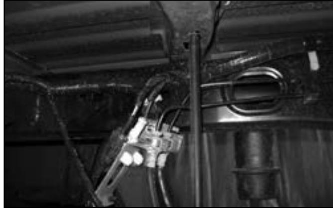
95. Attach the brake line to the relocation bracket with the 5/16" bolt, nut and washer (Bolt Pack #896 or #895). Torque to 15 ft-lbs. The brake line will need to be slightly deformed down to install into the new brake line bracket.
