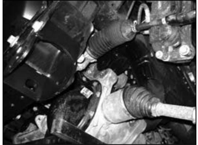
32. The rear bushing will need to be modified to provide clearance to the frame pocket. Use a hammer to dent the outer edge over on the bushing cup that is pressed into the front differential. (Fig 19A / B) Dent this over until the outer ridge is touching the aluminum housing. This will NOT affect the performance of the differential bushing, but will provide clearance to the frame.
