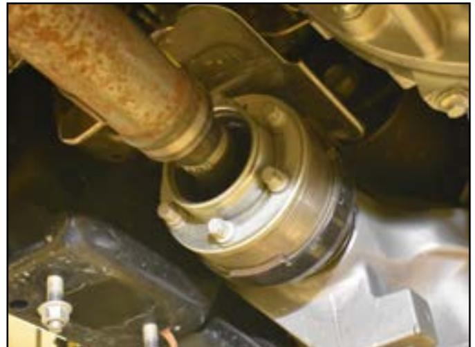
26. **Optional:** Remove the passengers side CV only. Strike the shaft with a hammer to dislodge it from the splines. This will make handling the differential much easier (Fig 14).
