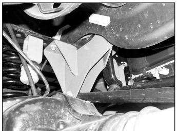
23. Pull the OE front bump stops free from the bump stop cups and remove the bolt mounting the cup to the frame (Fig 9).
