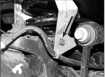
7. Remove the clips holding the front brake lines to the brackets on the frame. (Fig 2A) Using a proper line wrench, break loose the hard line at the junction block and rotate it 180 degrees. (Fig 2B) This will put the rubber line to the bottom. Tighten the hard line securely. Leave the brake line loose and save the retaining clip.
