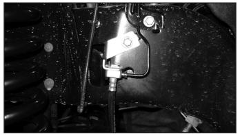
42. 6" Lift Only (013614): Remove the factory brake line brackets from the frame. Install the new provided brake line brackets and secure with the factory hardware. Carefully reform the brake hard line and install the junction block through the bottom of the new bracket. (Fig 15) Fasten with the original brake line clip.
