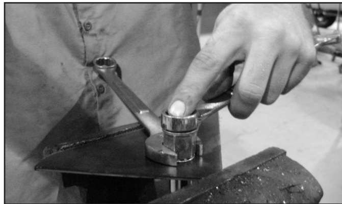
FIGURE 2 - 1/2" RIVET NUT SHOWN
