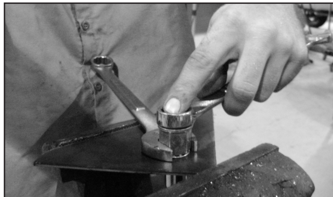
FIGURE 28 - 1/2" RIVET NUT SHOWN
