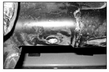
19. Place the machined sleeve into the existing frame rail hole. Reinstall the bracket with hardware (#793) and sleeve as shown (Fig 11a, 11b, 11c)
