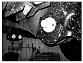
44. Turn the steering wheel to get the trackbar to align with the bracket. Install new 18mm bolt and tighten to 150 ft-lbs (#792).
