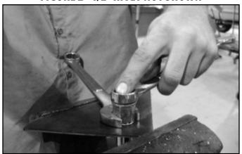
FIGURE 2 - 1/2" RIVET NUT SHOWN
