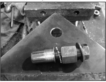
FIGURE 1-1/2" RIVET NUT SHOWN
