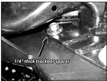
28. Fish the bolt tab through the frame rail with the included bolt wire and attach to the trackbar bracket with ½" USS washer and regular nut. Apply loctite to the bolt threads. Attach the upper hole with ½" x 1-3/4 (#792) bolt with spacer washer as shown. (Fig 15a, 15b)
