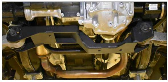
50. Install the new differential skid plate to the front crossmember with ½" x 1-1/4" bolts and ½" SAE washers (BP #480) into the welded nuts in the crossmember. Install the back of the skid plate to the rear crossmember with ½" x 1-1/4" bolts and ½" SAE washers (BP #480) into the welded nuts in the crossmember. Leave hardware loose. (Figure 24)
