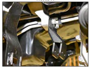
38. Install the two front driver's side front differential drop brackets so that the bracket without the lower cutout (03655) is toward the outside of the vehicle (offsetting out) and the one with the cutout (03656) is on the inside (offsetting in). Fasten the brackets to the frame with OE bolts with loctite into the factory threaded holes. Leave hardware loose. (Fig. 15)
