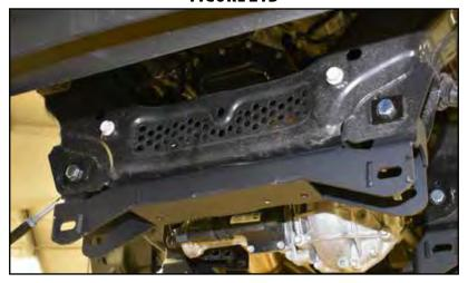
48. Install Sway Bar drop Brackets using OE hardware in the upper sway bar mounts (03931/03932) (Figure 22).
