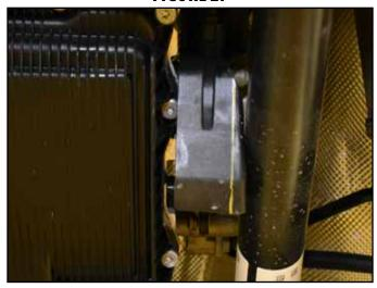
**56. Steps 54-57 are for the 6 inch kit only, For 4 inch kits, move to step 58.** In order to give a close to level stance after installation, preload spacers are included in these systems. Install the preload spacers if a more level stance is desired. The preload spacer will reduce the rake by an additional 5/8". Place indexing marks on the strut body, strut cap and upper coil seat (Figure 28 & 29) for realignment of the components when the strut is reassembled.
