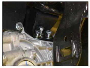
43. Attach the Passenger side differential to the bracket using 12mm x 60mm bolts and washers. (BP 480) (Figure 20)
