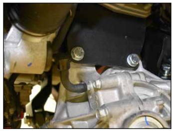
42. Attach the drivers side rear bracket to the differential with 12mm x 40mm bolts and washers (BP #480). Leave all differential hardware loose. (Figure 19).
