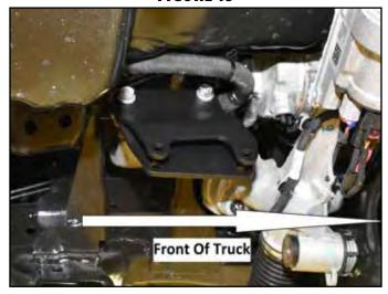
39. Install the driver's side rear differential drop bracket (03661) to the OE mount location with three 1/2" x 1-1/2" bolts and ½" SAE washers (BP #480). (Figure 16) The bracket will have the gusset plate towards the front of the vehicle. Leave hardware loose.
