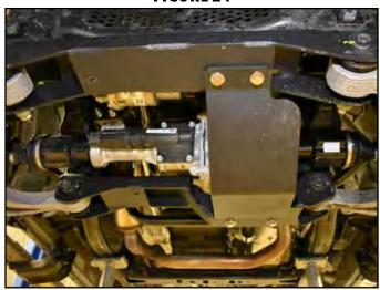
51. Install the lower control arms in the front and rear crossmembers. Attach the control arms to the crossmembers with the OE cam bolts, washers and nuts running from front to rear. Leave hardware loose. (Figure 25)
