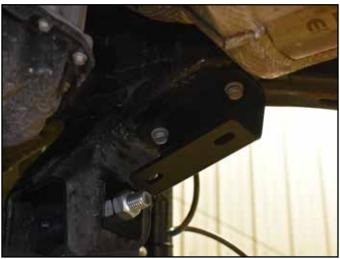
49. Install the new rear crossmember (01296B) in the OE rear lower control arm pockets and loosely fasten with the provided 18mm x 150mm bolts, nuts in conjunction with the provided cam slot washers (03982). Run the bolts from front to rear and leave loose at this time. (Figure 243
