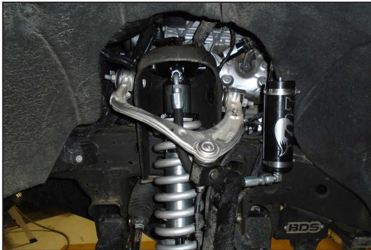
FIGURE 10 (NON DSC RESERVOIR - DRIVER SIDE)
