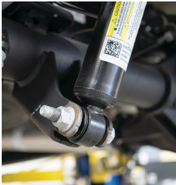
Fig. 25: Remove lower shock mount bolt.
