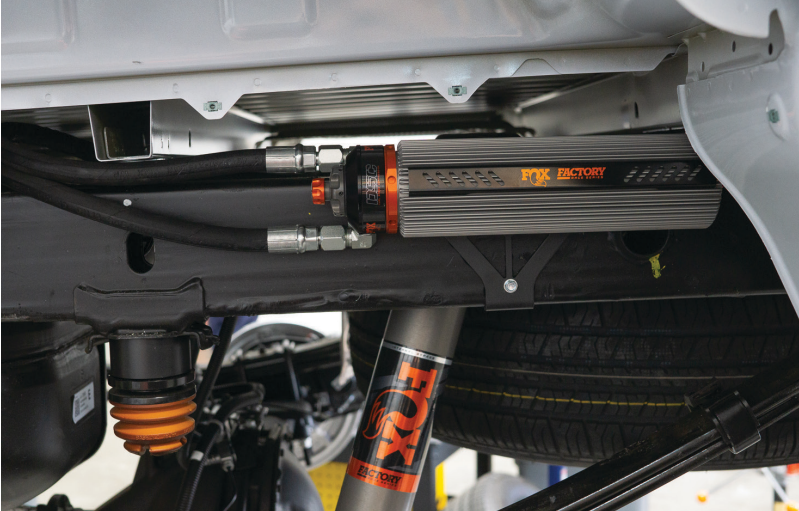
Fig. 38: Mount the reservoir.
