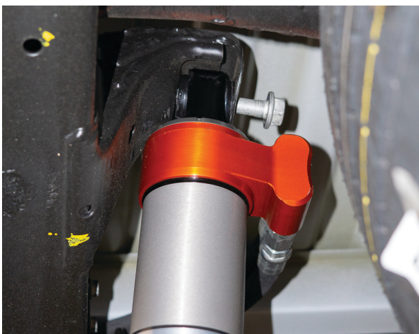
Fig. 33: The reservoir bridge faces inboard.
