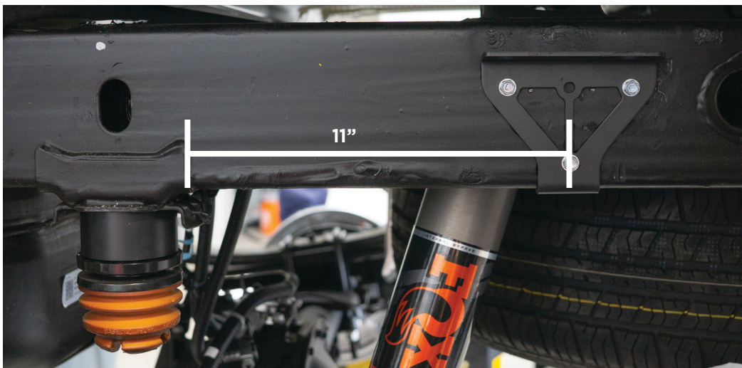
Fig. 37: Mount the reservoir bracket.
