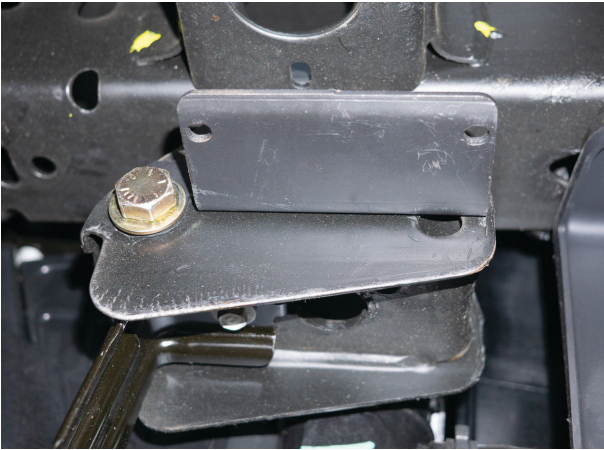
Fig. 11: Use the holes in the vehicles frame.
