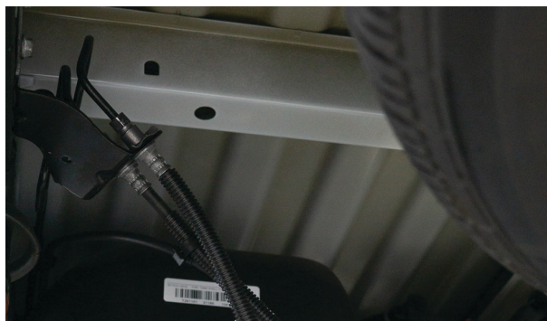
Fig. 27: Bend the brake line bracket.
