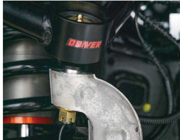
Fig. 18: Reattach UCA to the upright.
