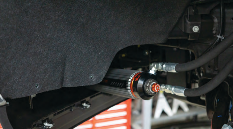
Fig. 23: Cut fender liner.
