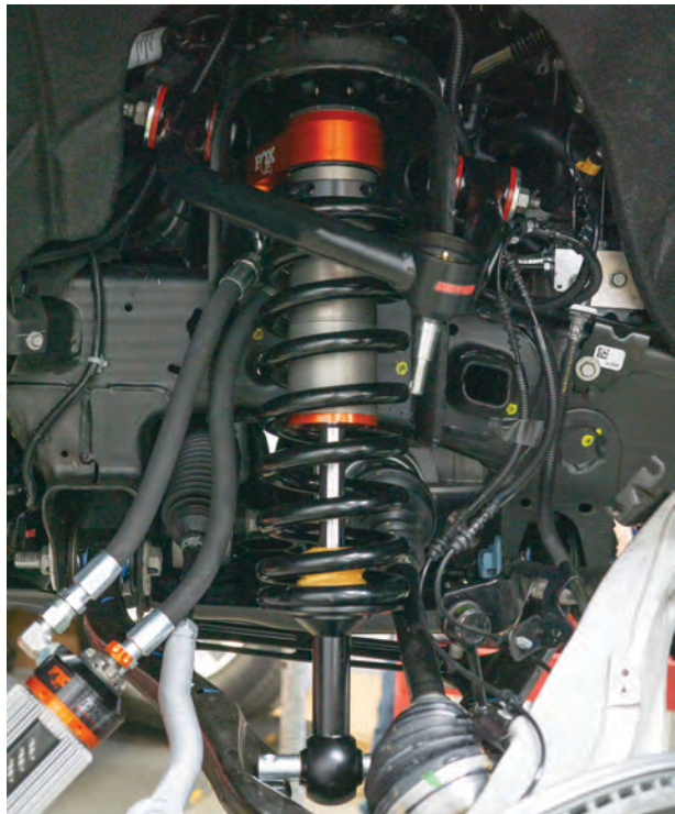
Fig. 13: Driver's side coil-over assembly is featured.
