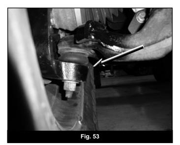
6. To determine the Z-height use the following equation: Y-X=Z. For the intended 7" of lift the value for Z should be approximately 4". If your value for 'Z' is less then 4" the torsion bars need to be adjusted up (tightened). If your value for 'Z' is more then 4" the torsion bars need to be adjusted down (loosened). These values are for reference but should not vary more then 1" in either direction.
