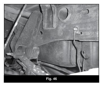
4. Disconnect the factory brake line bracket attached driver's side frame rail. The nut is accessed on the outside of the frame (Fig 47).
