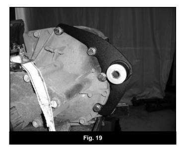
40. Locate the new passenger's side differential bracket (02192). Install the bracket on the existing studs on the passenger's side factory bracket. Fasten with the original nuts and washers. When installed the open side of the bracket will face inward and the bracket will taper down as it goes to the rear (Fig 20). Torque nuts to 65 ft-lbs.
