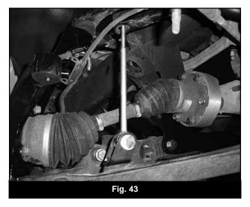
76. Install a provided stem washer (S100776) followed by a stem bushing (SB26BK) on each sway bar link. Install both links into the sway bar and install a second stem bushing followed by a second washer. Fasten the sway bar link upper assemblies with 3/8" nylock nuts (BP 569). Leave nuts loose (Fig 44).
