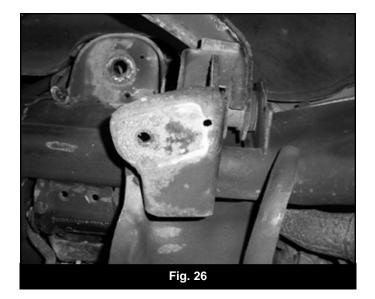
48. Locate the new provided bump stop brackets (02199). Place a bump stop bracket up to the original mount and line up the center of the two slots with the two holes in the factory mount. Using the third slot in the bracket as a guide, mark the center position to be drilled (Fig 27). Remove the bracket and drill a 7/16" hole at the mark.
