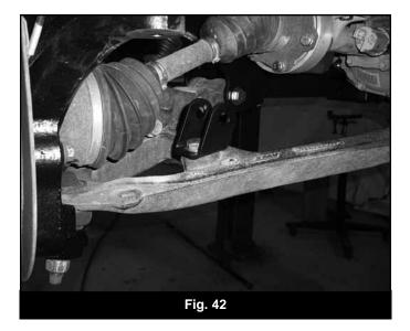
75. Locate the new front sway bar links (911109), small hourglass bushings (SB35BK) and 0.750" OD x 1.575" long sleeves (54587). Install the bushings and sleeves into the eyes of the links. Install the links into the new brackets on the lower control arms with 9/16" x 2-3/4" bolts, nuts and washers (BP 569). Run the bolts from front to rear and leave hardware loose (Fig 43).
