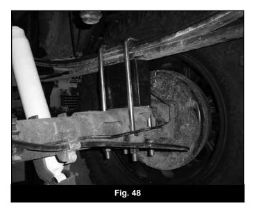
9. Repeat the installation on the driver's side of the vehicle. Pay special attention to all of the brake lines and wires. Do not allow them to get over-extended.
