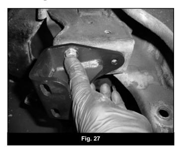
49. With the holes drilled, attach the new brackets to the frame with 3/8" x 1-1/4" bolts, nuts and 3/8" washers (BP 572). The two outer bolts should be all the way to the outer edge of the slots in the brackets (bracket push inward toward frame as far as possible). Torque bolts to 30 ft-lbs. Install the factory bump stop on the new brackets with the original mounting nut. Install the bump stop so it is offset toward the rear of the vehicle (Fig 28). Tighten bump stop hardware securely.
