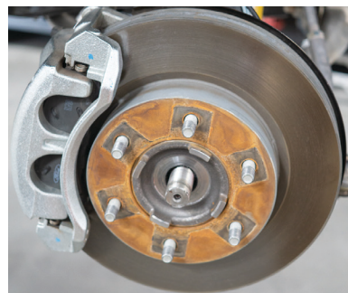
Fig. 7: Push the axle shank flush.
