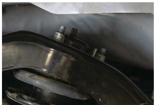
Fig. 27: Do not remove the center nut.
