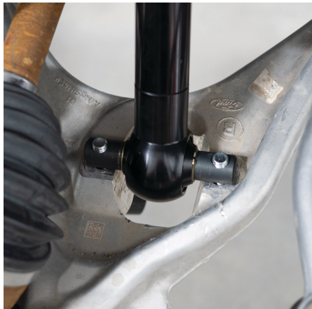
Fig. 15: Fasten the bar-pin bolts.
