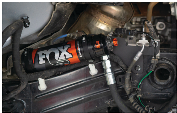
Fig. 16b: Mounted reservoir.
