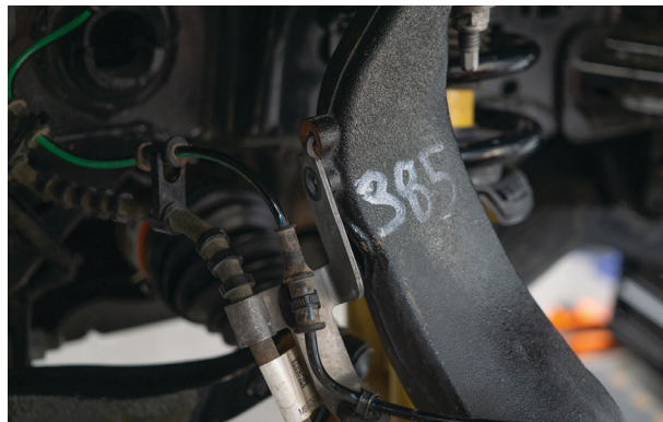
Fig. 4: Disconnect brake line bracket.
