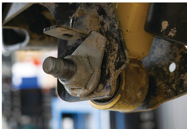
Fig. 26: Loosen the lower mounting bolt.
