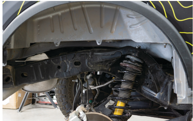
Fig. 24: Pull the fender liner.
