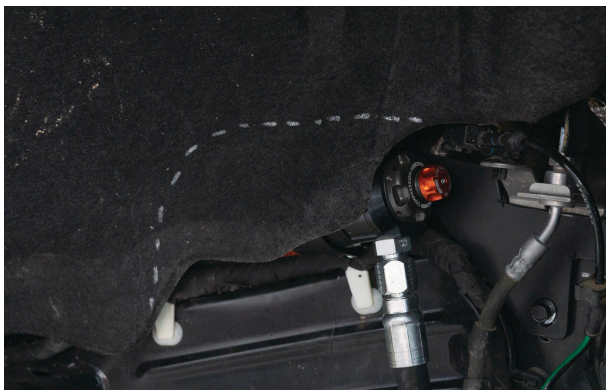
Fig. 22: Test fit the fender liner.
