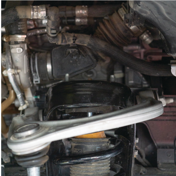
Fig. 9: DO NOT remove the center nut.
