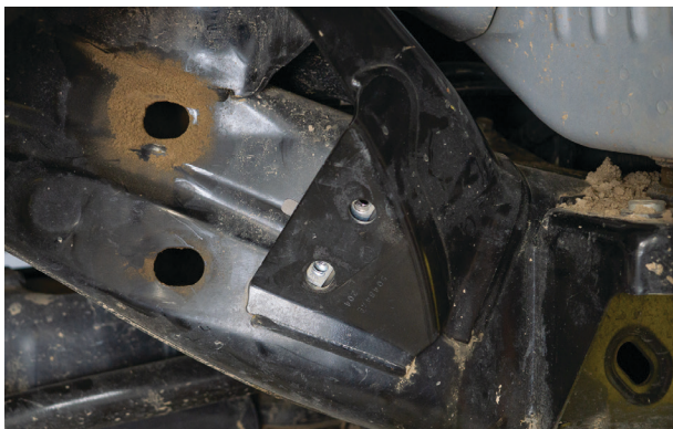
Fig. 30: Align backing plate with the frame.
