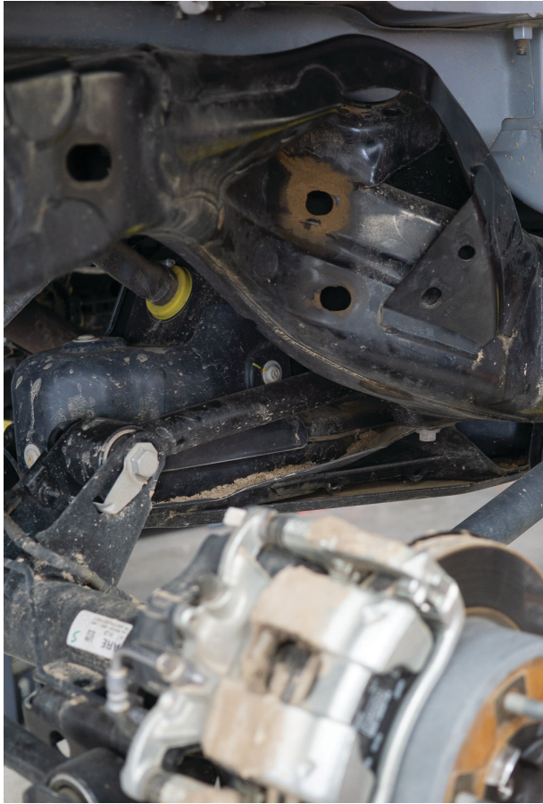
Fig. 28: Remove the stock coil-over.
