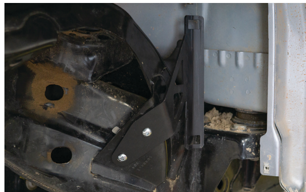
Fig. 31: Mount the reservoir bracket.
