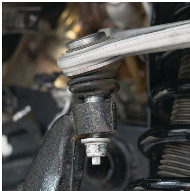
Fig. 8: Separate the UCA from the upright.
