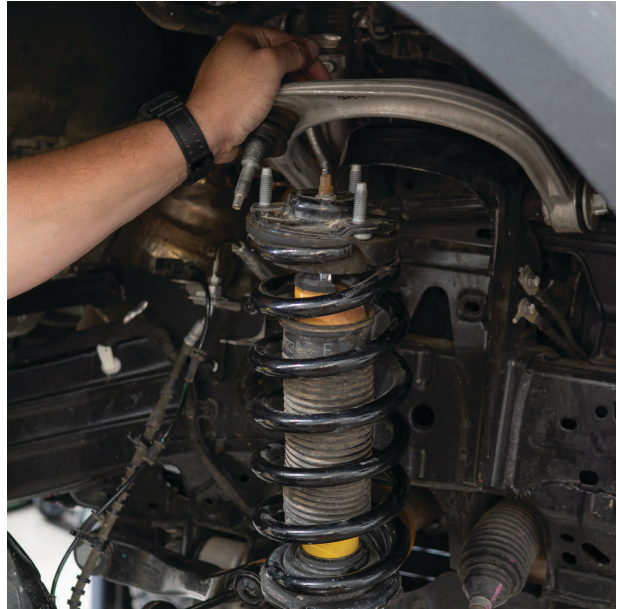
Fig. 10: Free the coil-over from the coil bucket.
