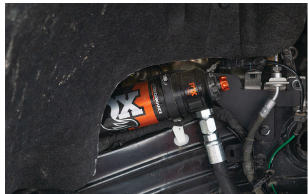
Fig. 23: Cut fender liner.
