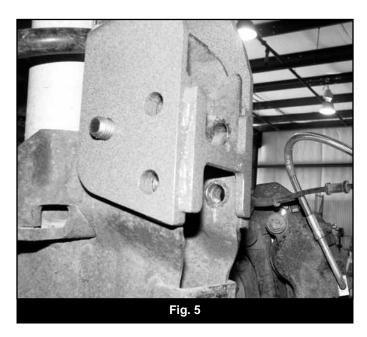
23. With all of the holes drilled, reattach the bracket to the axle and install the 9/16" x 5" bolt with 9/16" SAE washers and nut (bolt pack #614) in conjunction with the provided 7/8" x 2-3/8" spacer sleeve (72-1) placed in the OE upper control arm mount location. (Fig. 6) Leave hardware loose.
