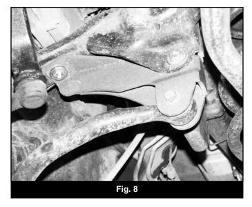
31. Apply loctite to the threads on the OE sway bar links. Thread the provided link extension (01249) on the OE links and tighten securely. Attach the extension to the sway bar with the OE washers, bushings and nuts. Tighten the nut until the bushings begin to swell. (Fig. 9)
