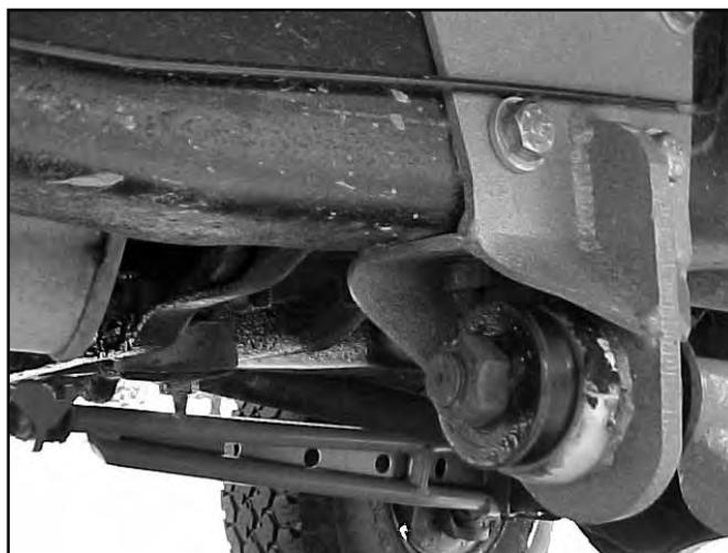
10. Raise bracket into position on the frame and secure with the 1/2" fasteners.
