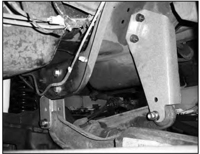
17. Tighten axle pivot drop bracket hardware as follows: 9/16" 110 ft-lbs, 1/2" 75 ft-lbs.
