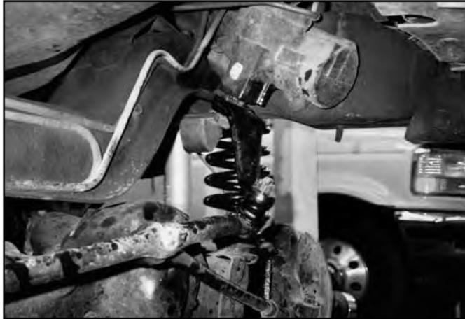
22. Place new BDS Coil Spring (4" or 6" lift coil spring) onto spring seat and secure with OEM fasteners. Raise assembly into the upper spring tower and secure with the OEM clip. (Fig. 12)
