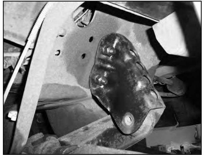
14. Cut out the template on the back of the instruction sheet. Place template as shown in the figure. Note: Match the holes to be drilled to the replacement bracket given in the kit. The two holes shown should be vertical, and the outer profile should be horizontal. Drill holes out to 9/16". (Fig 9)
