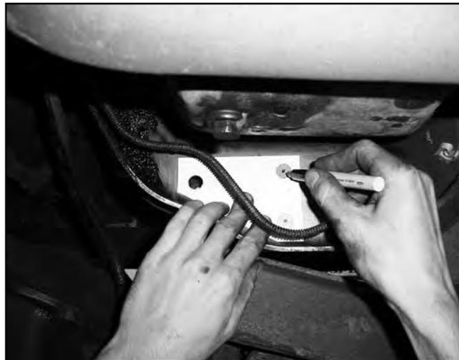
15. Install bracket with a new 9/16" x 3" bolt with nut and washers through the OE mounting hole. Attach bracket to drilled holes with 1/2" x 1-1/2" bolts with nuts and washers. Leave hardware loose at this time.
