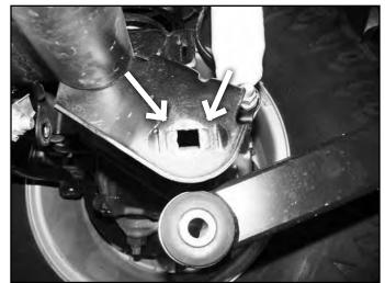
15. When the perforated sections are removed from the lower control arm mount, reinstall the control arm to the axle with the factory bolt with octagon washers with the bolt as far rearward in the slot as possible. Just snug the cam hardware so that the cam washers are retained within the stops. Final cam bolt torque will be completed with the weight of the vehicle on the suspension. (Fig 4)
