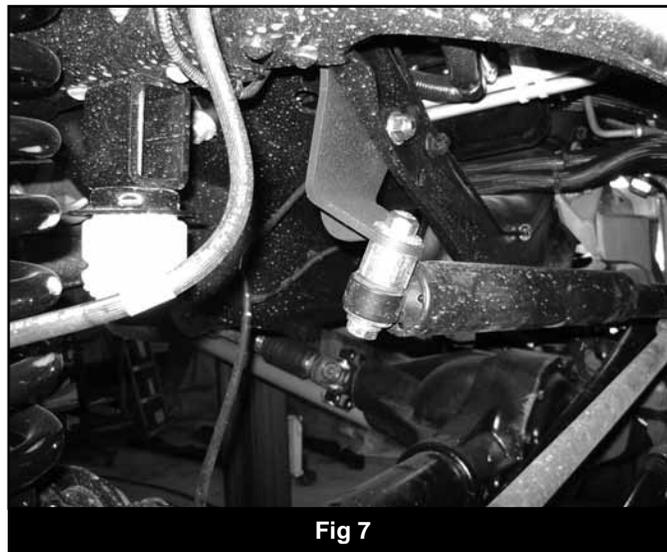
14. Disconnect the (5) bolts mounting the OE track bar bracket to the frame. Remove bracket and retain hardware.
