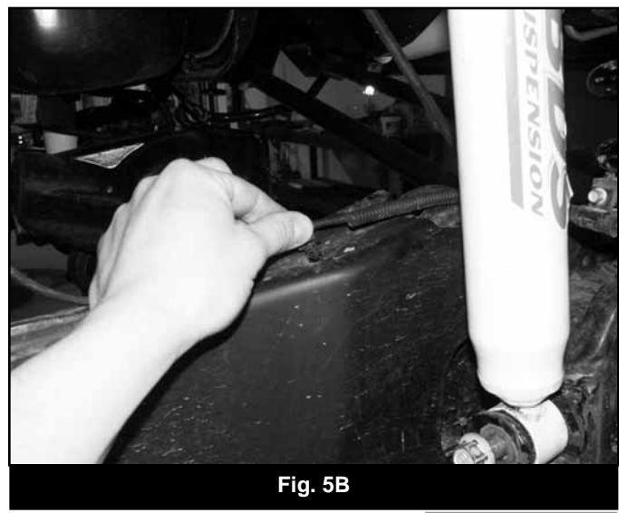
11. Disconnect the OE steering stabilizer from the frame mount.
