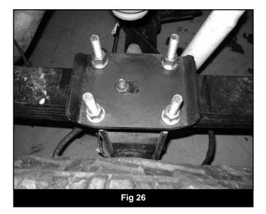
67. Repeat block installation of the driver's side. Take care not to over extend the brake lines. **Note:** *The parking brake cable bracket will need to be removed from the spring center pin. (Fig 26)*
