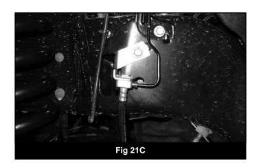
53. 6" Lift Only: Remove the factory brake line brackets from the frame. Install the new provided brake line brackets and secure with the factory hardware. Carefully reform the brake hard line and install the junction block through the bottom of the new bracket. (Fig 22) Fasten with the original brake line clip.
