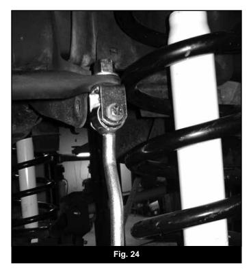
Models with y-link steering (03-08 models that have the drag link go from the pitman arm to the passenger's side steering knuckle). This steering does not provide enough clearance to the sway bar mounts, they must be modified. If you have an 03-08 model with the new T-link setup, installation of the brackets is still required due to the length of the sway bar links.
