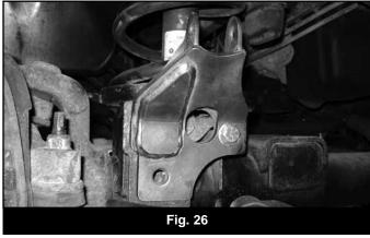
64. Repeat installation for drivers side. Align the bracket with the existing hole. Mark the opposite hole and drill both holes to  $\frac{1}{2}$ "-17/32". Reinstall the bracket with  $\frac{1}{2}$ " bolts (with loc-tite) with washers on the outside and square nuts on the inside of the bracket. Tighten to 65 ft-lbs. (Fig 27)
