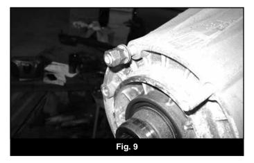
18. Install the transfer case indexing ring onto the transfer case. Note: This will only go on one way, rotate until the holes line up. Certain model years use metric hardware (BP# 937), earlier years use standard 3/8" hardware (BP# 933). Match up the threads from the removed studs to ensure proper hardware is selected and attach with counter sunk allen bolts with loc-tite on threads. Ensure the ring goes on square and there are no gaps. Tighten to 35 ft-lbs. (Fig 10).
