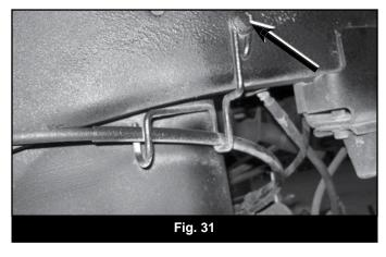
85. Disconnect the parking brake cable by unthreading nut with 13mm ratchet wrench.
