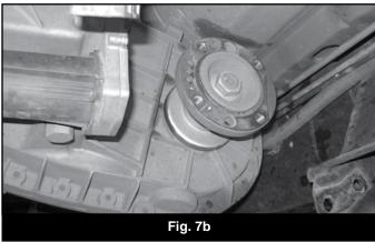
14. Support the transfer case and remove the 6 nuts that attach the transfer case to the transmission. (Fig 8a, 8b)
