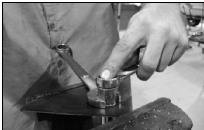
FIGURE 2 - 1/2" RIVET NUT SHOWN
