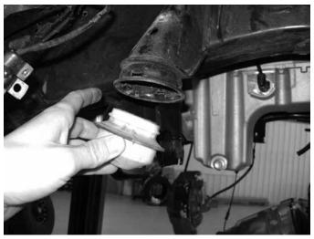
37. Clearance the hole inside the bump stop cup to 11/16", a step drill is highly recommended, if one is not available, a rotary die grinder can be used. Insert and seat ½" rivet nut. Follow rivet nut installation at the end of the instruction sheet. (Fig 25)
