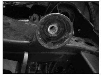
38. Attach the new bump stop extension (02813 – DRV, 02814 – PASS) to the rivet nut with ½"x 2" hardware (use socket and extension to attach) and to the cross member with ½"x 1-1/4" bolt, washers, and nut. (BP #683) (Fig 26)
