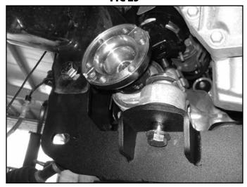
35. Reconnect the differential breather line and the central axle disconnect wiring harness.
