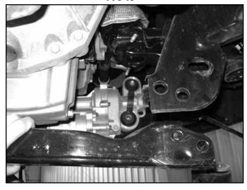
23. Support the differential with a hydraulic jack (transmission jack preferred). Remove the remaining two front mounting bolts and lower the differential from the vehicle. (Fig 16)
