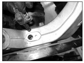
13. Remove the CV nut. CV's have a tight fit to the hubs, it may be necessary to use an air hammer to separate them. Reinstall the nut a few turns to keep from damaging the CV shaft if this method is used. (Fig 6)
