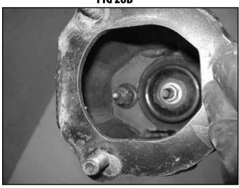
43. Install the strut and spacer into the vehicle. Attach the strut to the upper mount with new 3/8" nylock nuts and washers (BP #943). Attach lower mount to the lower control arm with factory bolts. Tighten the 3/8" hardware to 35 ft-lbs, do NOT tighten the lower mount at this time. It will be done at the end of the installation with the vehicle weight on the ground. (Fig 29a, 29b)
