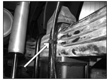
86. Use two zip ties, secure the e-brake cables together in front of where the old e-brake cable guide bracket contacted the cables. (Fig 47)
