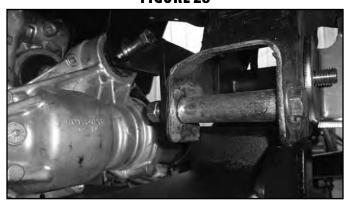
41. Install the differential to the new driver's and passenger's differential brackets. Loosely attach the differential to both differential drop brackets with 9/16" x 4" bolts, prevailing torque nuts, and washers (Fig 29C & D). The passenger's side differential bracket will use a spacer (03622) on the front side between the bushing and the differential bracket (Fig. 29A & B).
