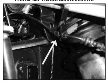
68. Attach the front sway bar to the sway bar drop bracket with the provided 3/8" bolts, prevailing torque nuts, and washers (Fig. 43). Attach the sway bar link to the front control arms. Torque the 3/8" bolts for the sway bar drop to 37 ft-lbs. Torque the sway bar link to the lower control arm to 74 ft-lbs.
