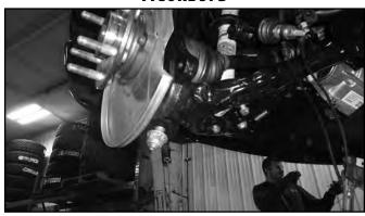
58. Attach the knuckle to the upper control arm with the original upper ball joint nut (Fig. 38).
