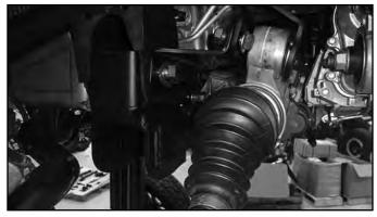
43. Install the 9/16" x 4" bolts, prevailing torque nuts, and washers in the rear cross member and through the differential mount on the rear cross member (Fig. 31). Leave hardware loose.
