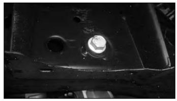
25. Remove the nut from the passenger's side differential mounting bolt (Fig. 19A). Carefully lower the differential to the ground while removing the long bolt for the passenger's side differential mount (Fig. 19B).
