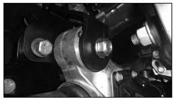
42. Install the new rear cross member (03616) with the provided longer 18mm bolt, prevailing torque nuts, and washers. The tabs on the cross member should align with the center diff. bracket. Run the bolts from front to rear. Leave hardware loose. Make sure the passenger's side bolt runs through the differential brace. (Fig. 30).
