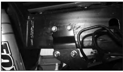
18. Install the provided ABS line bracket to the top of the rear differential using the factory mounting hole and factory bolts. The bracket will rotate the ABS line 90 degrees facing up. Attach the ABS line bracket to the relocation bracket with two 1/4" x 1" bolt, prevailing torque nut, and washers. Torque the factory and 1/4" bolt to 8 ft-lbs. (Fig. 7)
