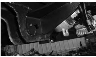
37. Install the front cross member (03615) in the control arm pockets with the the provided shorter 18mm bolt, prevailing torque nuts, and washers Run bolts from front to rear (Fig. 25). Leave hardware loose. Make sure to attach the differential bracket to the frame on the driver's side with the provided hardware.
