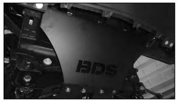
52. Install the provided strut spacers on the strut with the provided 10mm prevailing torque nuts and washers. The spacers will only install one way (Fig. 35). Torque hardware to 30 ft-lbs.
