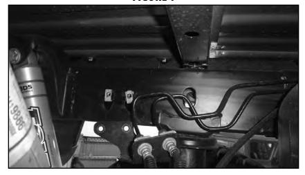
5. Remove bolts attaching the ABS lines to the top of the rear differential (Fig. 2).
