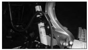
5. Remove the ABS sensor from the steering knuckle (Fig. 2).
