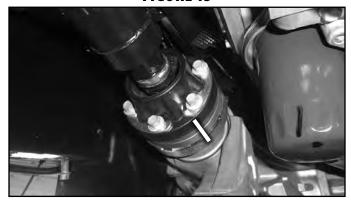
20. Remove the bolt attaching the differential to the rear cross member (Fig. 14). The hardware will not be reused.
