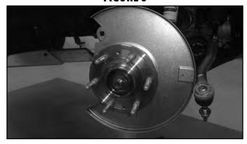
11. Remove the sway bar links nut from the the lower control arms (Fig. 7). Save the hardware.
