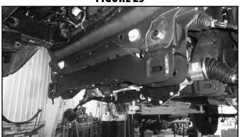
38. Install the new passenger's side differential bracket (03731) to the original mounting location with the new 14mm bolt, 14mm washer, and factory nut (Fig. 26). Snug up hardware, but do not tighten.
