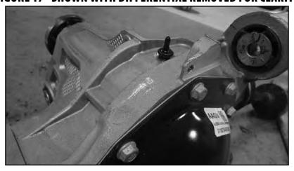
24. Support the front differential with an appropriate jack. Remove the driver's side differential mounting bolts (Fig. 18). Save mounting bolt hardware.
