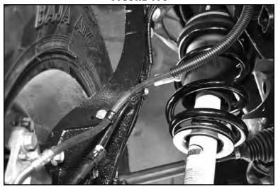
67. Attach the ABS wire and brake sensor wire the the upper control arm on the driver and passenger sides with the relocation bracket (03673 & 03674) and factory hardware using thread locker. The passenger side will use the lower hole of the relocation bracket (Fig. 42).
