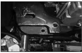
32. The bottom front of the front lower control arm pockets must be cut to provide clearance for the front cross member. This area needs to be cleaned of any oil, grease and/or undercoating. These coatings are flammable.
