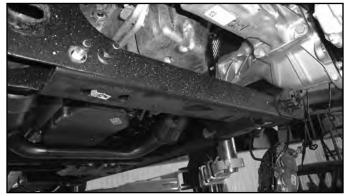
Disconnect the differential actuator wire connector from the actuator (Fig. 16).
