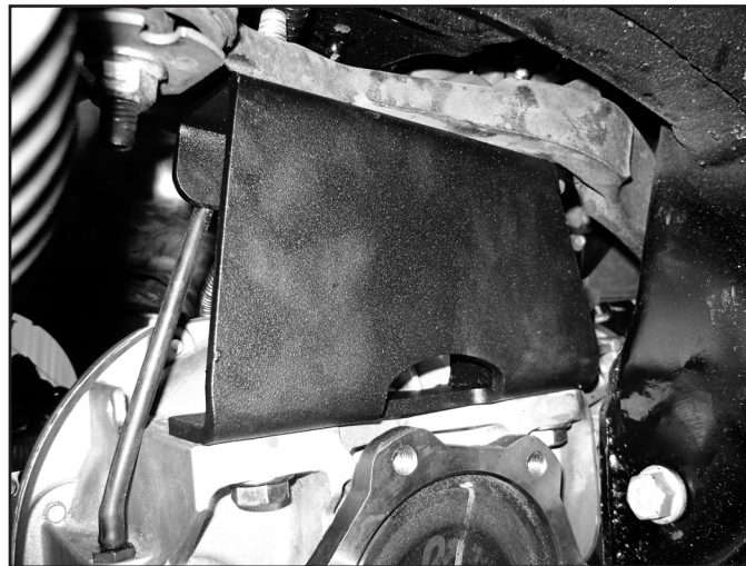
FIGURE 27 - SHOWN WITH DIFFERENTIAL ALREADY INSTALLED
