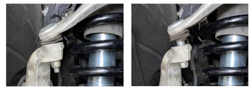
G. Remove the upper ball joint from the spindle and carefully secure the spindle using a bungee to avoid tension on the brake line and ABS line.
