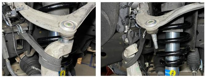
H. Using a 15mm socket/wrench, remove the two bolts securing the shock to the lower control arm.
