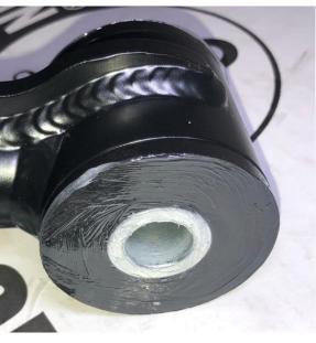
P. Install the 4 provided 90° zerk fittings into the threaded holes on the bottom of each bushing eye-ring ensuring they face outboard for easy access during service.
