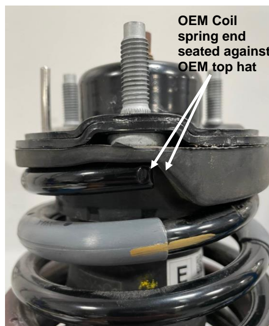
Figure 3: OEM Coil spring clocking. Damper module depicted above is without Badlands trim level or Sasquatch package
