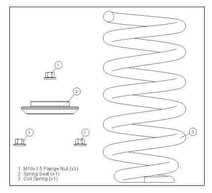
Fig 3: Bilstein supplied components
