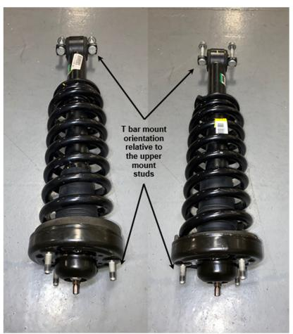
Figure 2: OEM T Bar Orientation
