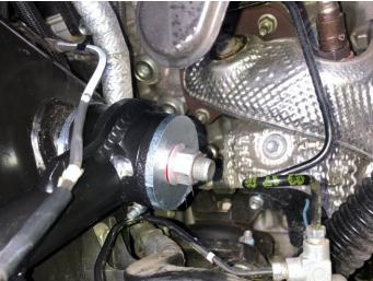
s. Install UCA ball joint on the spindle and secure using castle nut provided. Torque castle nut to 110 Nm (81 ft.lbs.) Continue to tighten the castle nut to the next available slot (no more than 60°). Never back off the slotted nut to achieve alignment with the hole in the stud. Install the cotter pin.
