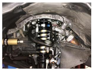
G. Using two 19mm wrenches, remove the nut and washer securing the UCA bolt.
