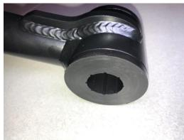
O. Apply the supplied grease to the bushing inside diameter.
