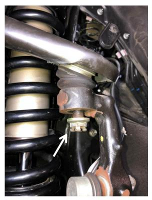
E. Using a ball joint puller, separate the spindle from the ball joint stem. Be careful to avoid tension on the brake line and ABS line.
