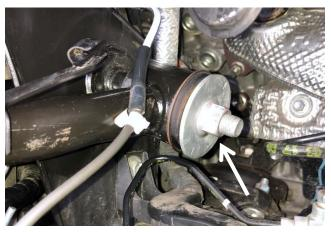
H. To allow removal of the driver side UCA bolt, locate the bolt securing the Main Wiring Harness to the Inner fender in the engine compartment below the battery. Using a 10mm wrench remove the bolt and secure the wiring harness out of the way.
