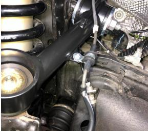
Using a 19mm socket and 19mm wrench, torque UCA bolt and flanged nut to 115 Nm (85 ft. lbs.).
