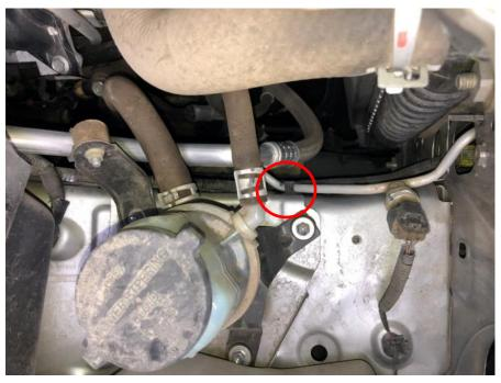
J. To allow removal of the UCA on both sides, remove the 2 clips that secure the smaller wiring harness to the inner fender.
