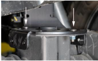
27. Place the 4 Air Bag Bracket Stand Supports onto the lower airbag bracket and sandwich them with the upper bracket/ airbag assembly. The whole assembly should seat together at this point.
