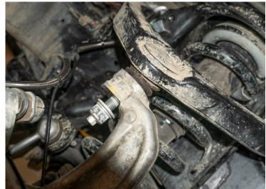
11. **Performance 2.5 ONLY** — 21mm — Remove control arm hardware from the frame and remove the factory control arms from the truck. Keep the hardware as it'll be reused with the Carli Arms.
