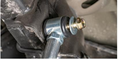
46. Use the provided lower 1/2" bolt and crimp lock nut with a washer between the bolt head/sway bar and bushing/nut to secure the link to the inside of the sway bar. Torque to 60lb.ft.
