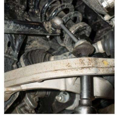
5. 21mm — Remove the Tie Rod Ends from the knuckle. Loosen the nuts until they're only engaged a few threads. Use a tie-rod end puller to disengage the tapers. Once it drops, remove the tie rod end from the housing.
