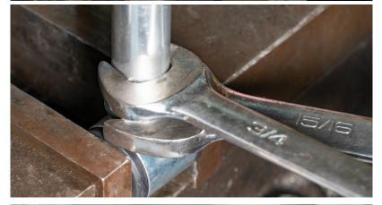
45. Use the provided M10 x 60mm upper bolt and fender washer to assemble the end link the welded frame nut. Torque to 30lb.ft.
