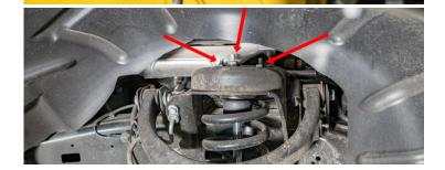
21. Performance 2.5 ONLY — Insert one of the provided grade 8 bolts and a washer to start the outermost upper control arm thread in the top of the coilover. USE Anti-seize as you're threading grade 8 bolts into aluminum threads!
