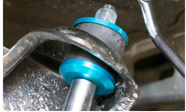
42. For the 2019+, you'll need to install the smaller crush sleeve into the upper end link bushing (10mm ID). The 14mm ID sleeve can be pressed out in a vice or hammered out. We use a vice with an 11mm deep socket to press out the sleeve without disturbing the bushing assembly, then a larger piece of tube on the other side of the sleeve to receive it. The new sleeve should be greased and can be installed with the light tap of a hammer.
