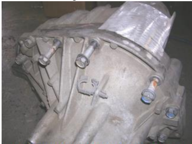
Figure 1: Clean up excess material left from previous mount
