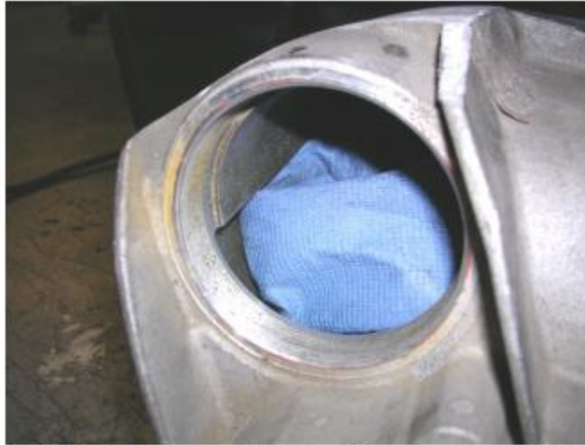
Figure 3: Vent cap removed, protect internals very carefully.
