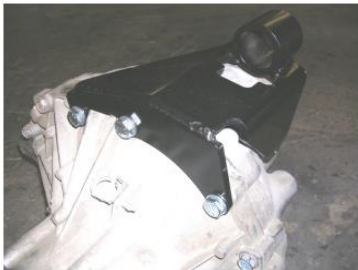
Figure 2: Installing the Cognito Bracket
