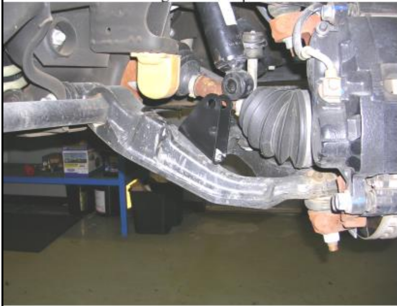
Figure 1: Cognito lower shock bracket installed
