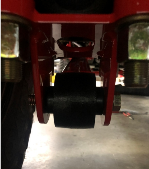
Figure 34: Traction Bar Rod End / Rear Axle Pivot
