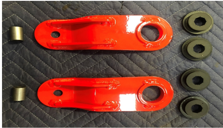
Figure 14: Traction Bar Shackle Parts
