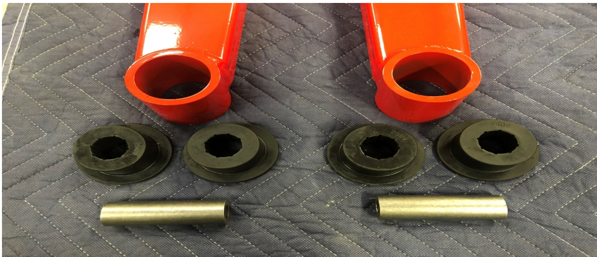
Figure 27: Traction Bar Bushing Parts
