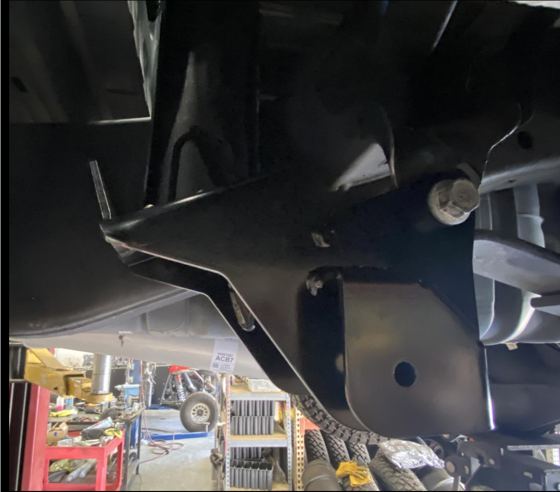
Figure 9: Assembled, welded, and painted mounting bracket.
