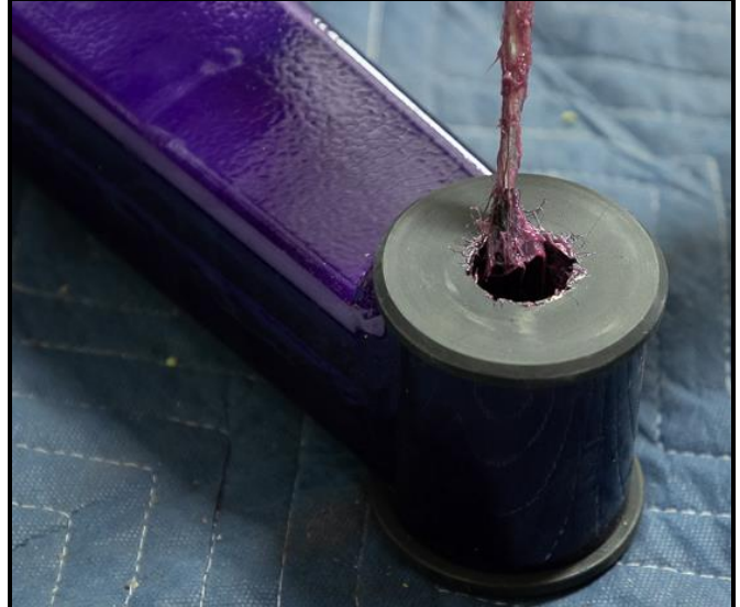
Figure 17: Traction bar bushing grease application.
