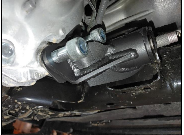
Figure 12: M14 bolts. Use washers here.
