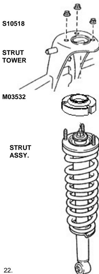
1. Read complete instructions before beginning installation, the following special tools are recommended: Coil spring compressor, floor jack, ball joint separator, jack stands, bench vise, and metric hand tools.
