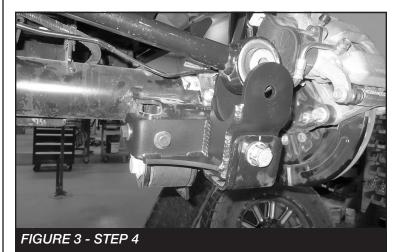
5. Install the track bar to the new Fabtech bracket using the supplied 5/8" hardware. Torgue to 170 ft-lbs. SEE **FIGURE 4**
