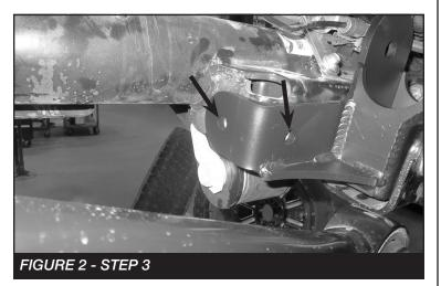
4. Reinstall the new Fabtech bracket using the factory bolt and the supplied 7/16" hardware. Torque the factory bolt to 160 ft-lbs and the 7/16" hardware to 65 ft-lbs. SEE **FIGURE 3**
