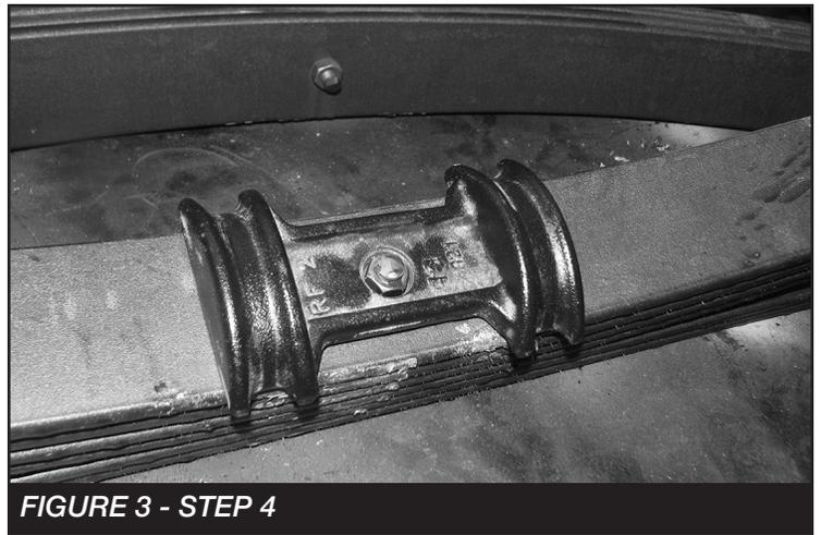
5. Install the new leaf spring into the original spring location using the factory shackle and hanger bolts. Torque to 148 ft-lbs. Use the supplied u-bolts to secure the new leaf spring to the axle. **NOTE: The factory block will be reused in the factory location.** Torque the u-bolts to 179 ft-lbs. **SEE FIGURE 4**
