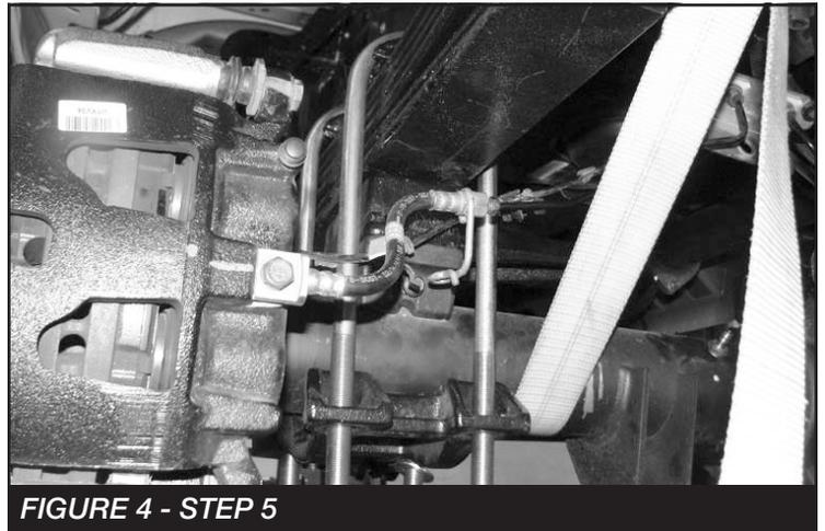
6. (11-UP MODELS) Locate the factory brake line mount on the driver side of the axle. Remove the vent line from the bolt and remove the bolt. Save hardware. Locate the supplied brake line bracket FT30059 from the front box kit and attach the side with the sleeve to the axle using the factory hardware. Using the supplied 3/8" x 2" bolt, nut and washer, attach the brake line to the other end of the bracket. Reattach vent line. **SEE FIGURE 5**
