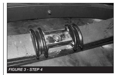
Install the new leaf spring into the original spring location using the factory shackle and hanger bolts. Torque to 148 ft-lbs. Use the supplied u-bolts to secure the new leaf spring to the axle. NOTE: The factory block will be reused in the factory location. Torque the u-bolts to 179 ft-lbs. SEE FIGURE 4
